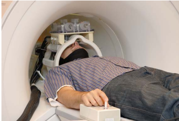
Figure 3. Sebastian, just before fully entering the scanner, with the MagLink 64-ch. EEG cap, the Avotec binocular video display & eye camera, and the 2-D joystick (all MR-compatible).
